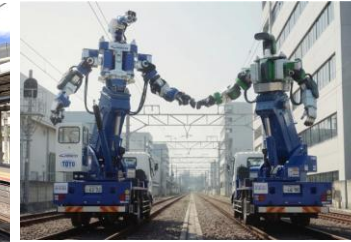
Multi-purpose railway heavy machinery ZIZAI
